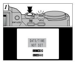
Press the "O" (Power) button to switch the camera on and off. When you switch the camera on, the indicator lamp turns green. If the date has been cleared, a confirmation message appears.
